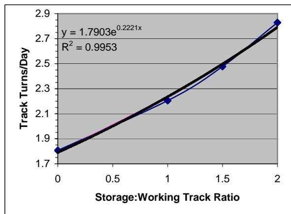
Figure 4.3 depicts the operational differences between 2:1, 1:1 and 0:1 storage to working track ratios. Based on this analysis, which confirms the industry rule of thumb, the Port should provide at least 1:1 and preferred 2:1 ratio of storage to working track at each of their on-dock rail yards.
